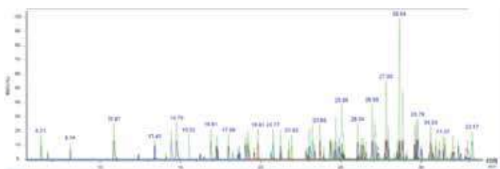
Chromatograms of 208 Pesticide Residues (A Group) Analysis by GCMSMS
